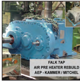
Air Preheater Rebuild
